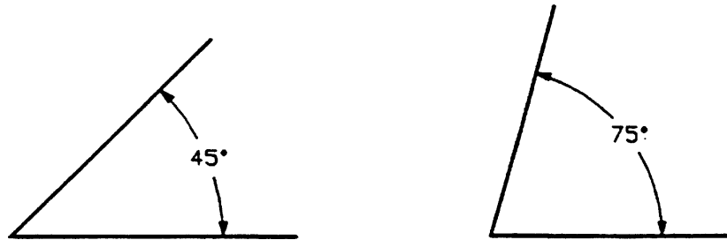
Fig. 5-5 POLYLINE CONTROLLED BY AN ANGULAR DIMENSION
